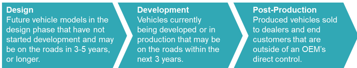
FIGURE 2 – VEHICLE LIFECYCLE PHASES
