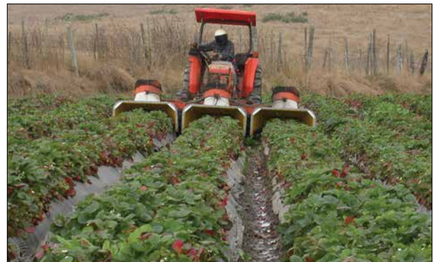
Figure 5. Tractor-mounted vacuum used to remove lygus bugs from strawberry rows. (C. Pickett, CDFA)
