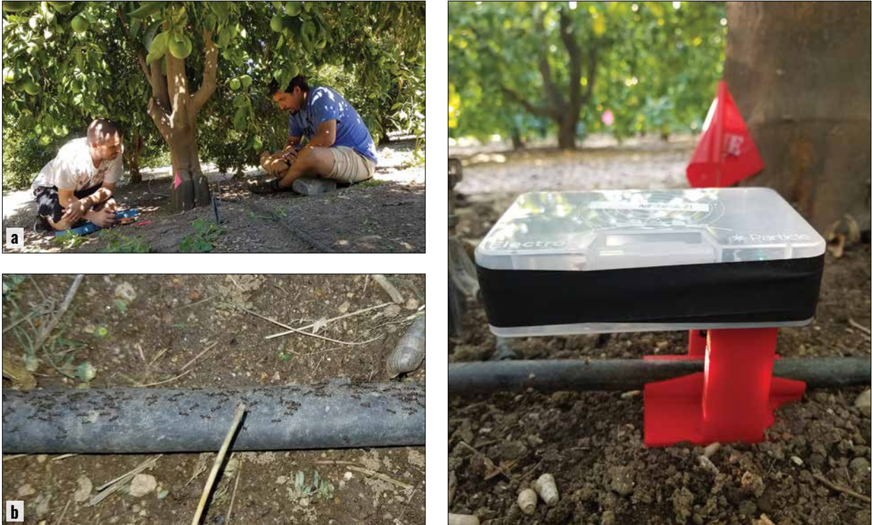
Figure 7. (a) Visually estimating L. humile densities ascending trunks of citrus trees; (b) Argentine ants using irrigation pipes as highways to move from subterranean nests over uneven soil terrain to tree trunks; (c) an infra-red sensor attached to an irrigation pipe with a 3D-printed clamp. (a–c: M. Hoddle UC Riverside)
