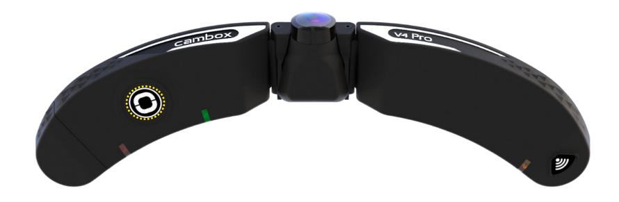
Press 1 second the On/Off button of your camera. Once the Power LED starts blinking green, press briefly the On/Off button again to pause the camera. The Power LED turns solid red.
