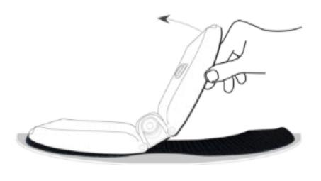
Once the first wing is detached from its velcro support, accompany the unfastening process of the Cambox by applying the same vertical and circular effort.
