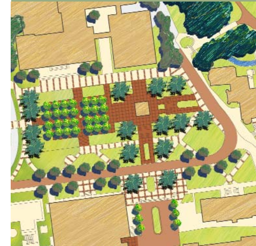
The Campanile Environs initiative converts South Hall Road and Esplanade Drive into pedestrian malls and upgrades paving, lighting, site furnishings and planting.
