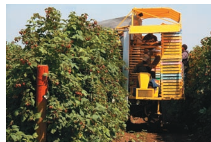
Oxbo 9000 over-the-row raspberry harvester
