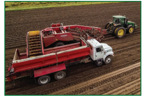
Potato harvesters are complicated machines that must dig the potatoes out of the ground, separate potatoes from other plant material, dirt, and rocks. Harvesters must do all this while being gentle enough to prevent bruising.
