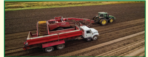
Potato harvesters are complicated machines that must dig the potatoes out of the ground, separate potatoes from other plant material, dirt, and rocks. Harvesters must do all this while being gentle enough to prevent bruising.
