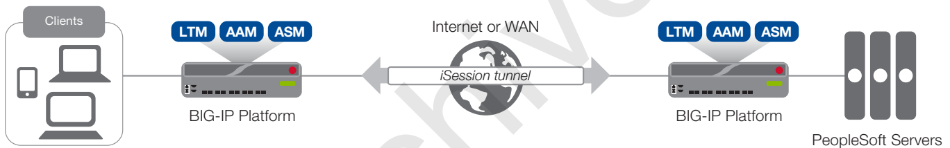
Figure 1: Using an iSession tunnel to secure and optimize traffic between two BIG-IP systems
