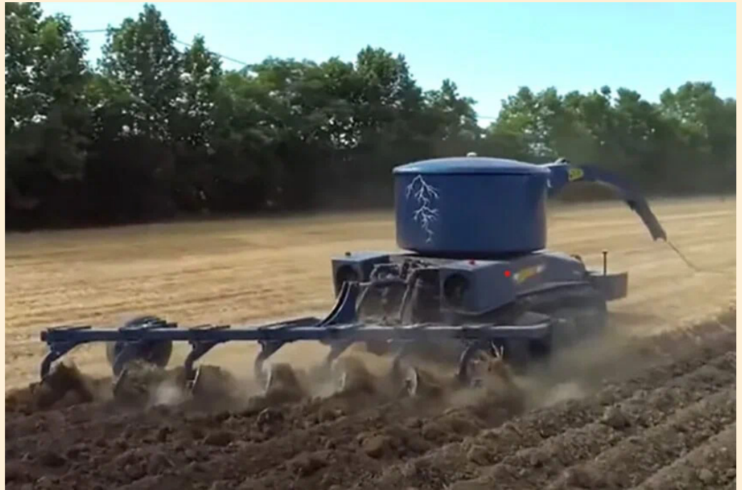
Source: Italians develop autonomous electric tractor with tethered power supply - Future Farming
