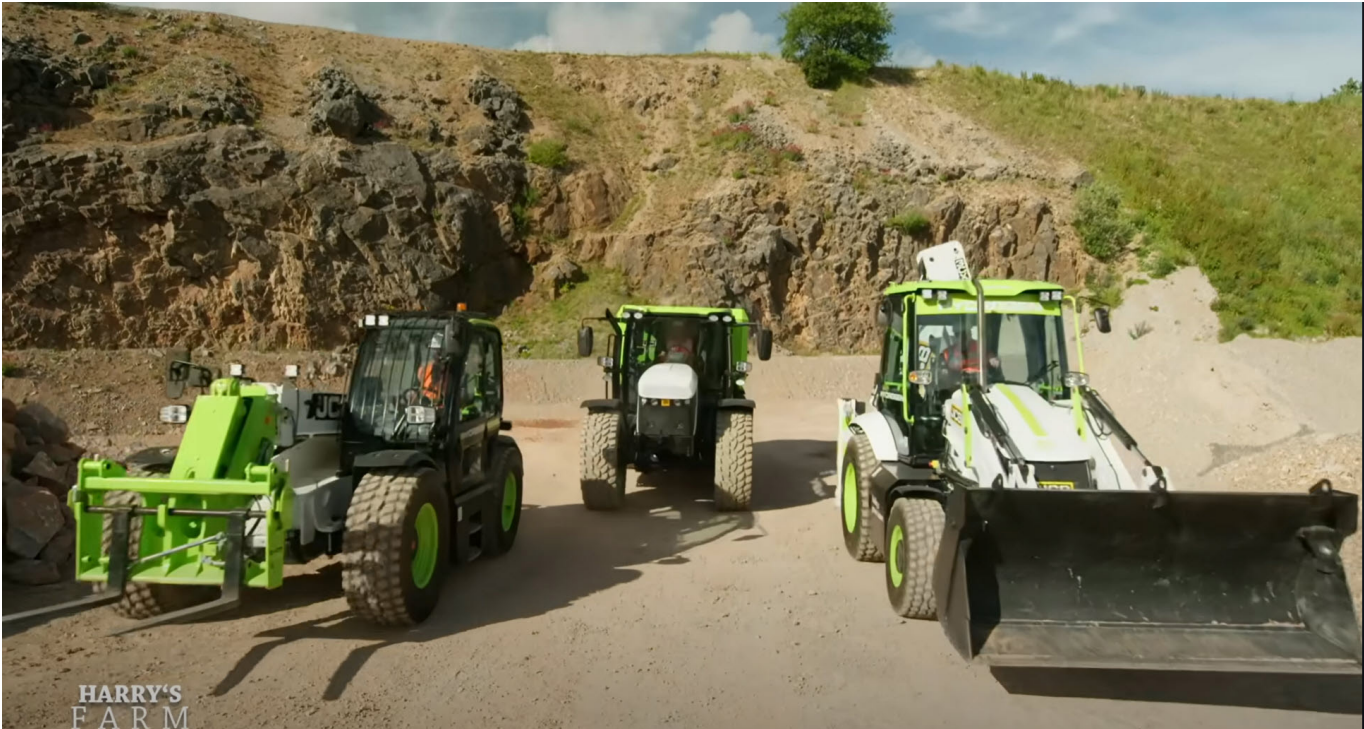
Below: JCB's Fleet of Internal Combustion Hydrogen powered machinery (youtube.com)
