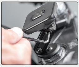
4. Set the Arm to your desired angle. Tighten both Arm Screws to lock the Arm in place. Max torque: 4 N•m.
