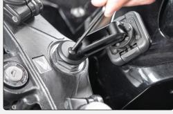
3. Place the Stem Mount in the steering stem. Tighten Base Screw with the Hex Key. Max torque: 4 N·m.
