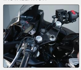
1. The **Stem Mount** is compatible with hollow steering stem nuts, typically found on clip-on style handlebars. If applicable, remove the plastic cap on your stem or replace the closed top nut with an open top nut.
