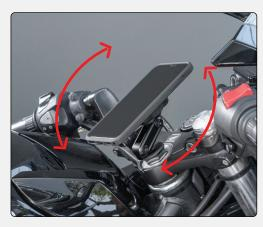
5. Before riding, slowly turn handlebars fully left and right with and with phone mounted to confirm no interference with nearby components (e.g. gas tank, fairings, gauges) Reposition and recheck if necessary.
