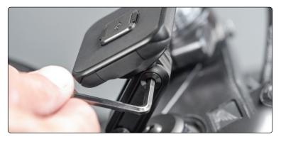
Warning! Screws may loosen over time due to vibration. Periodically check screw tightness.
