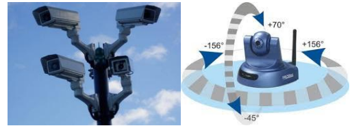
Figure 2: Examples of video surveillance cameras having the same position but different fields of view
