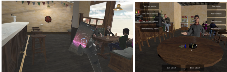
Fig. 3. The two implemented environments, a bar (left) and coffeeshop (right). Left, the implementation of one of the 6Ds: Declare —grabbing a phone to make a call in the virtual bar. Right, the therapist can alter the environment in a step-by-step way by using the ‘show element’, ‘move to location’, and ‘start and stop the tutorial’ buttons.
