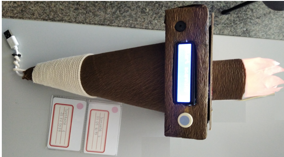
Figure 1: The Magic Torch prototype with two smart cards for the gaming question configuration.
