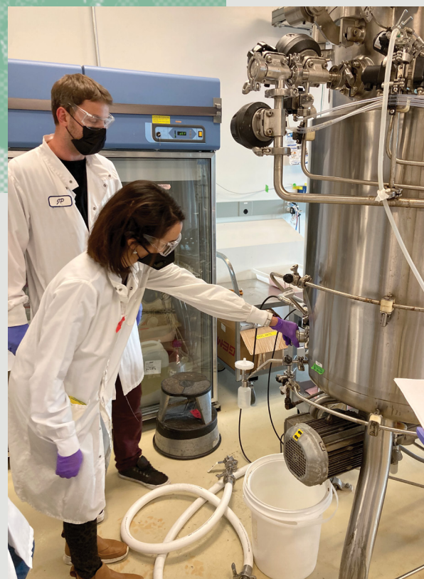
Vicky Olivares (front) with ABPDU Principal Process Engineer Jan-Philip Prah (back) take a fermentation sample from ABEC 300L stainless steel bioreactor.
