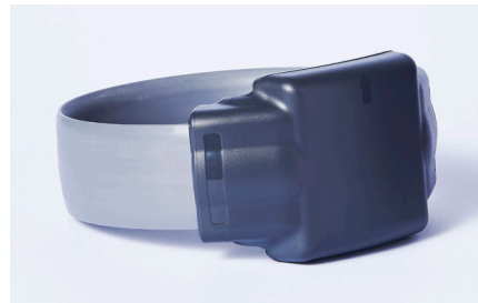
Example: Buddi’s SmartTag at 4 oz is an example of a smaller and lighter device design.
