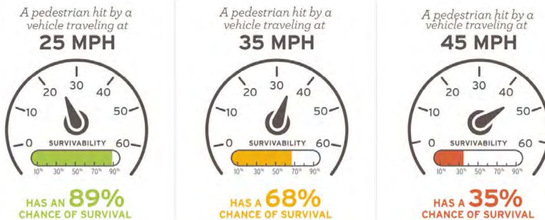
Impact speed and a pedestrian's risk of severe injury or death (Tefft 2011)
