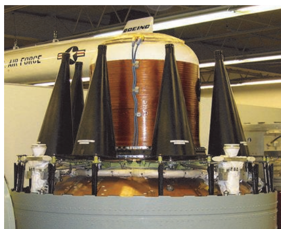
Conical nuclear warheads around the 3rd stage of a Trident C4 missile. D5 has a similar arrangement.
