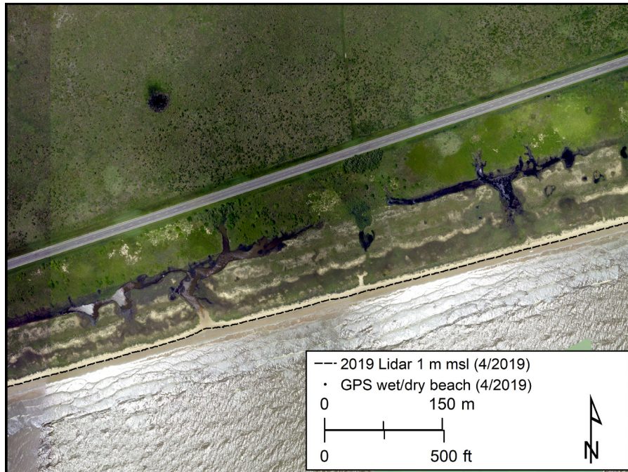
Figure 11. Shoreline position comparison on the upper Texas coast at Sea Rim State Park (SRSP, fig. 4). The 1 m (3.3 ft) msl shoreline proxy extracted from spring 2019 lidar data is superimposed on 2019 Bureau imagery.
