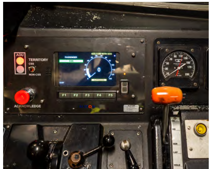
When a train passes over this device (top photo), Positive Train Control communicates with the cab system (bottom photo) to ensure safe operations.
