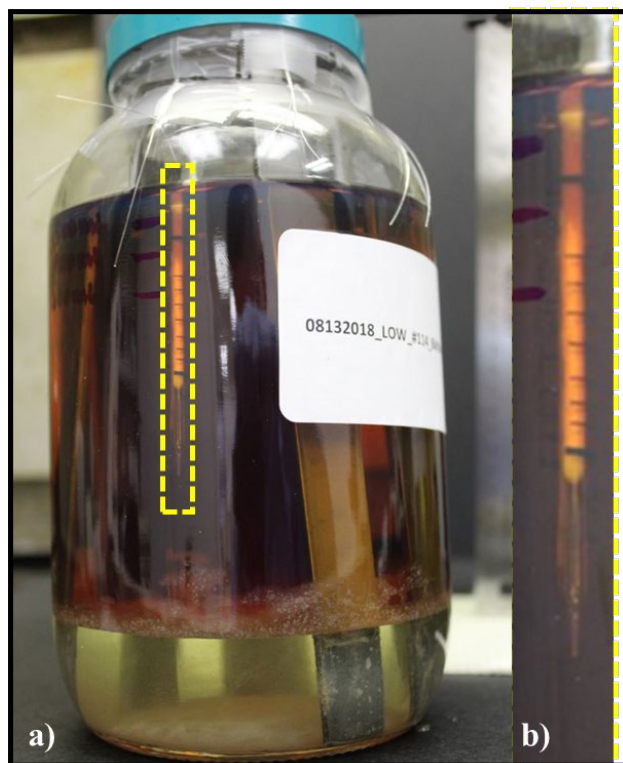
Figure 7. Positioning of Dräger tube in three-phase microcosm – a) Dräger tube in microcosm 114 showing inlet positioned approximately 3 cm above fuel-aqueous-phase interface; b) close-up view of Dräger tube.
