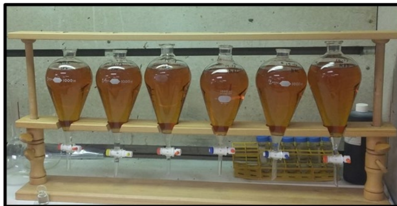
Figure 1. Partitioning experiment with 99:1 fuel to water ratio, after 24h.
