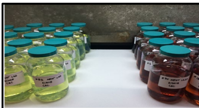
Figure 3. Partial view of test microcosm array – Right: LSD microcosms; Left ULSD microcosms.
