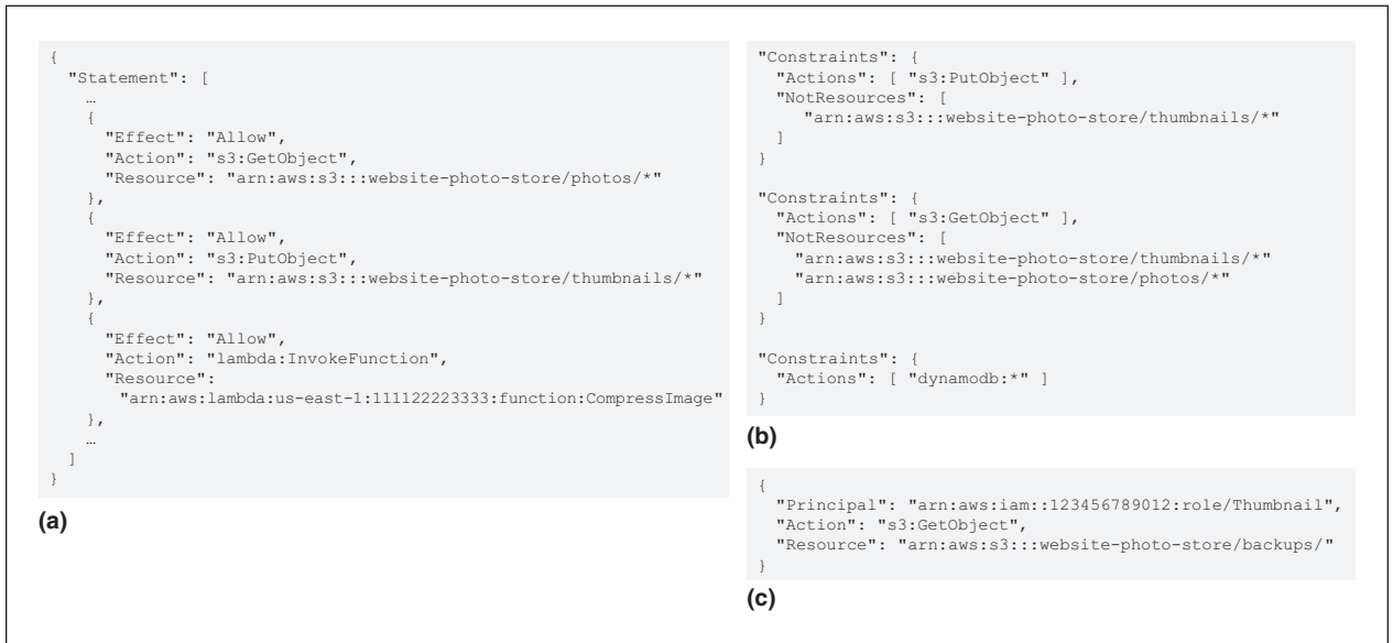
FIGURE 2. The policies and constraints in Zelkova: (a) a small portion of the access control policy for the Thumbnail Service from Figure 1, (b) three constraints representing violations of requirement 4, and (c) a representative violation report.
