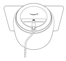
To give Echo Show 10 room to rotate, place it at least 15.5 cm from a wall. If you need to place it near a wall, don't worry—it can learn to adjust its rotation range.
