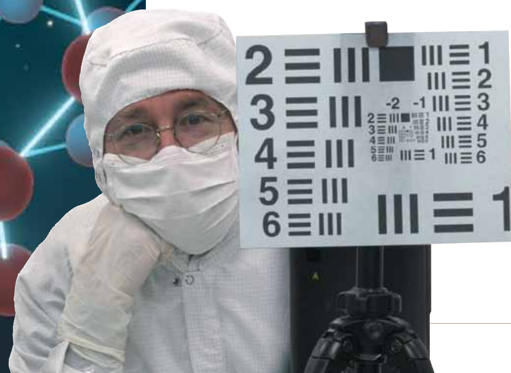
One of Curiosity’s cameras took an “eye” test after delivery to JPL (it passed). The standardized test target is used to measure optics systems’ resolving power as a function of contrast.
