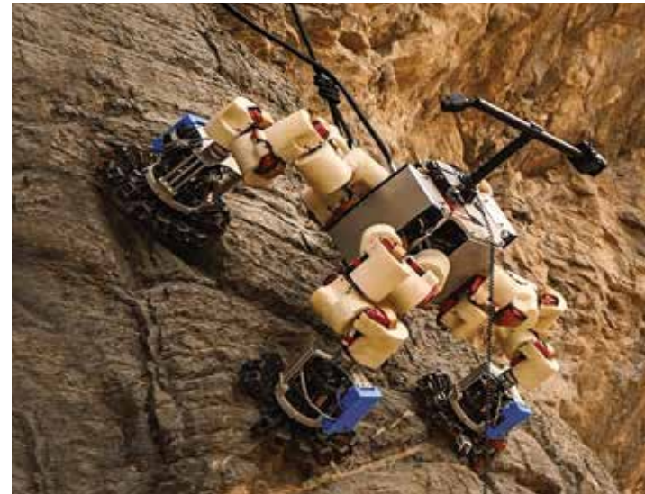
∇ LEMUR / Limbed Excursion Mechanical Utility Rover.
