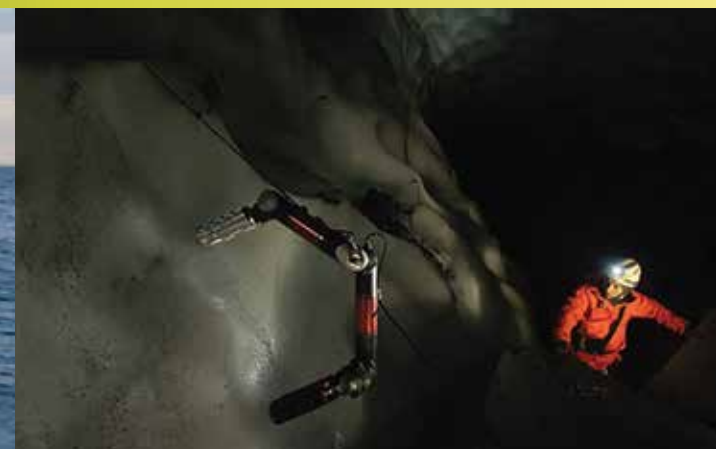
< Field testing the Ice Worm prototype in a glacier cave.
