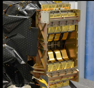
Above: JPL detectors shown integrated on Euclid's Near Infrared Spectrometer and Photometer instrument
