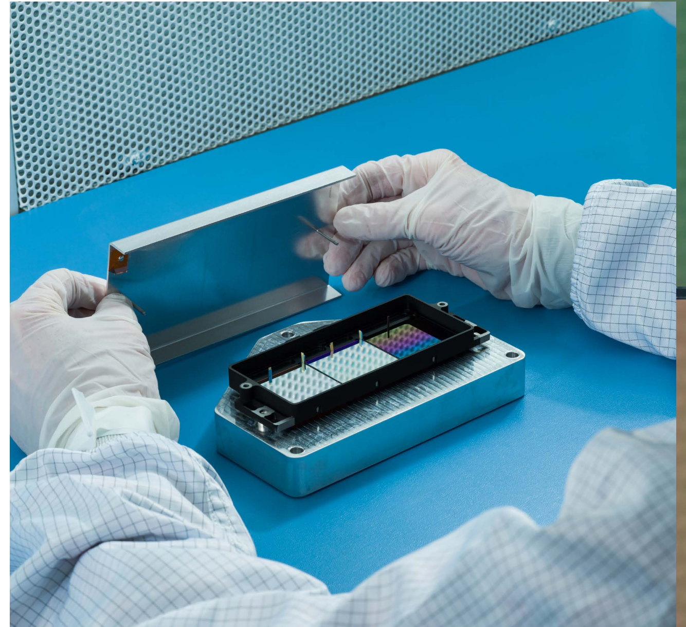
Above: A scientist assembles SPHEREx's Medium Wave InfraRed focal plane array.
