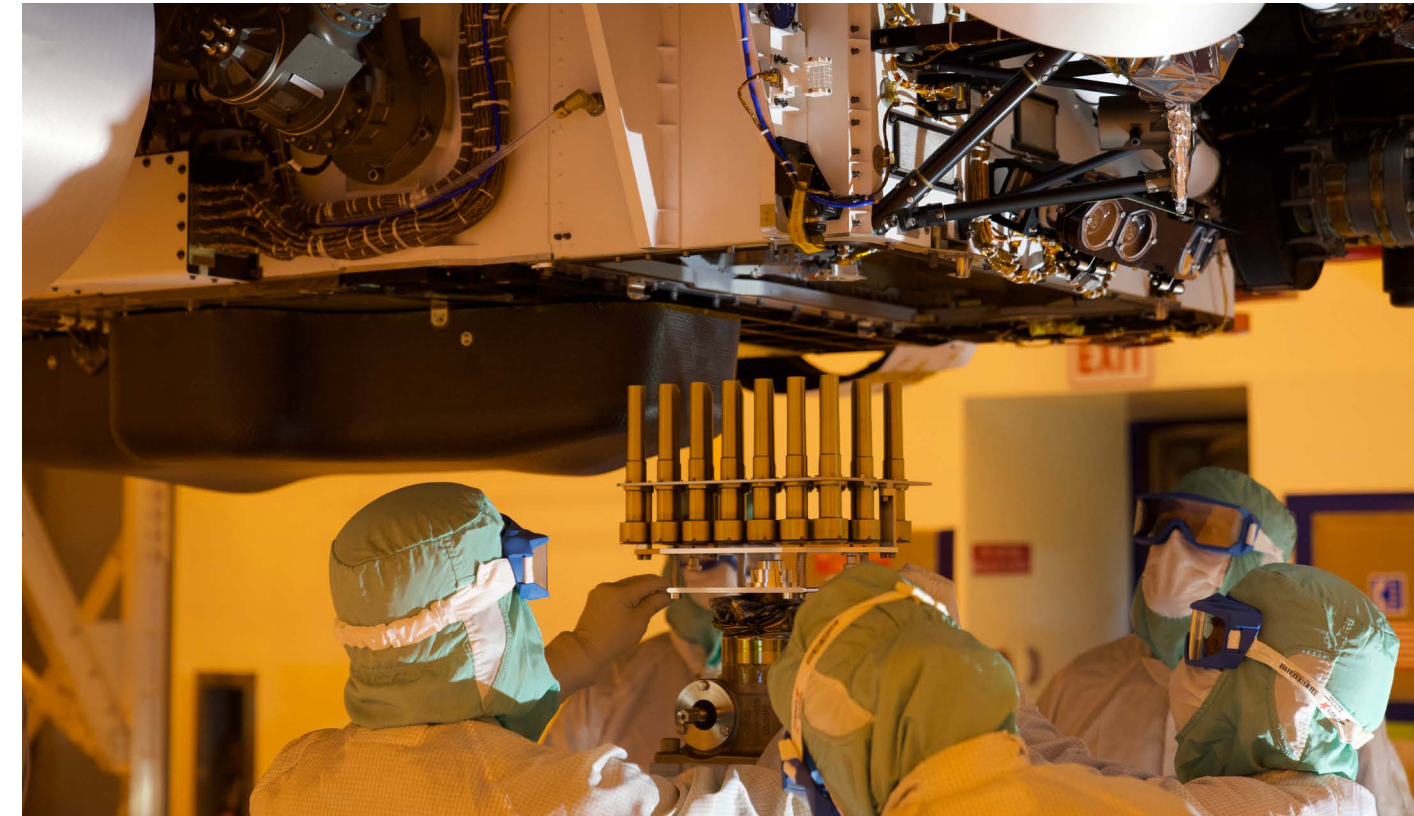
Above: A tray holding 39 of the 43 sample tubes was installed into the Perseverance rover before its journey to Mars in May 2020.
