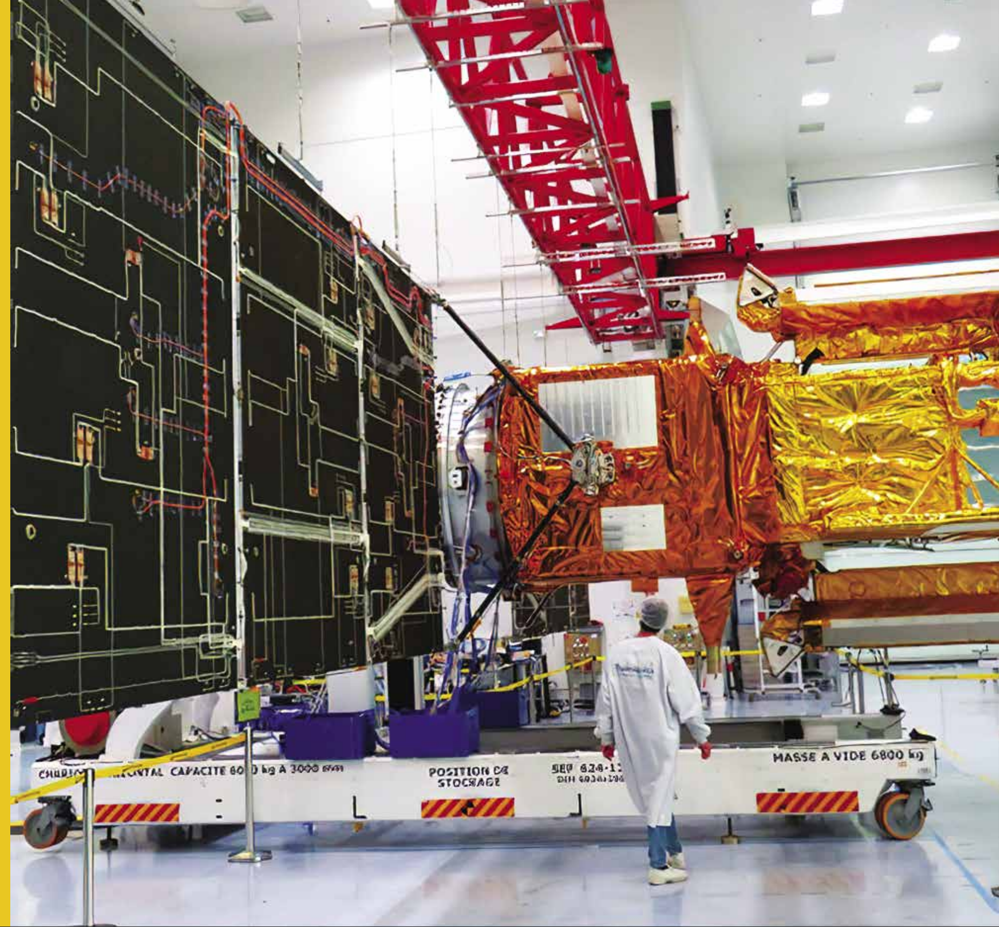
With its solar panels deployed, the SWOT spacecraft undergoes its integration and test engineering phase.
