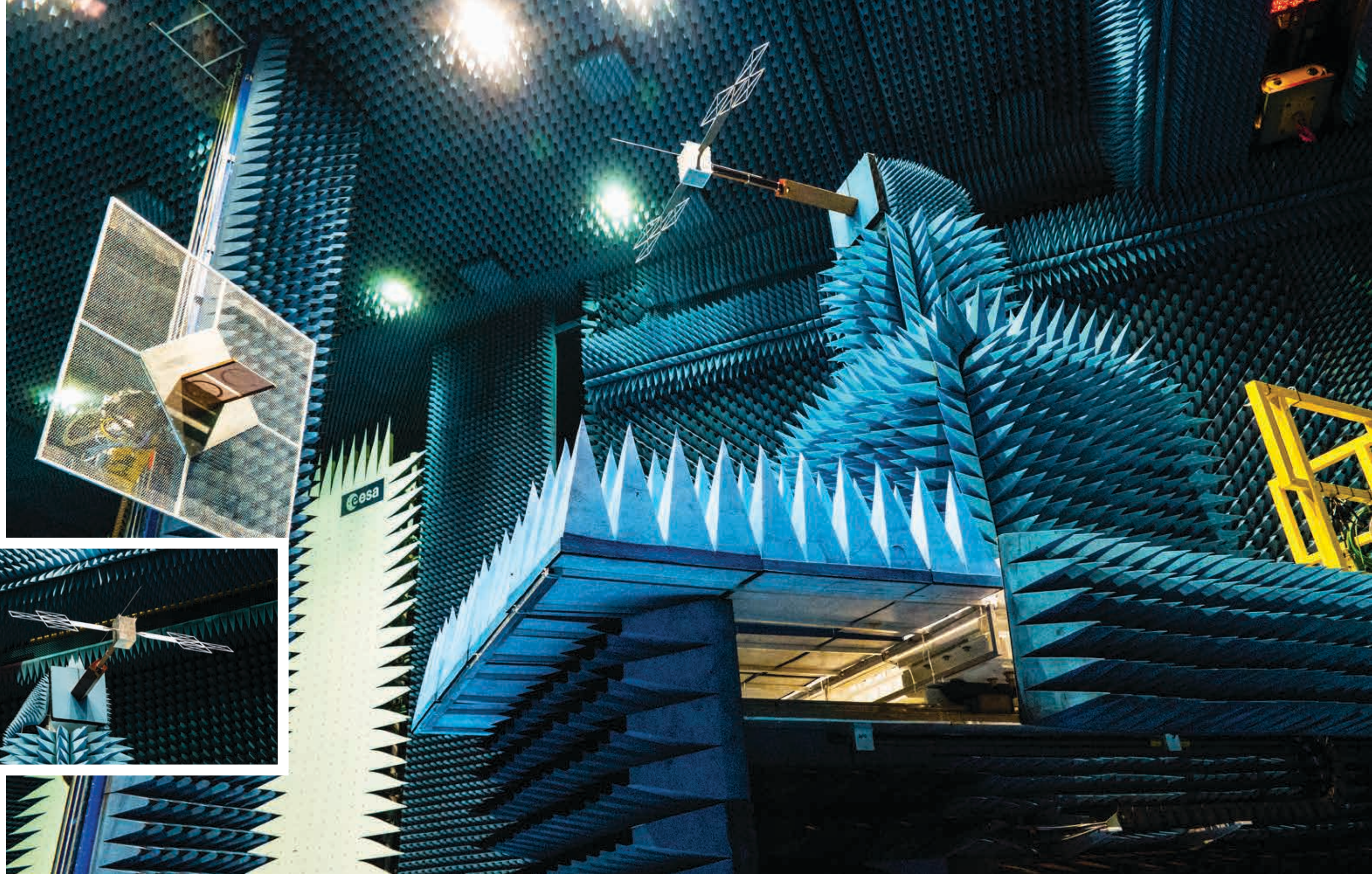
A scale model of JUICE's RIME antenna – Radar for Icy Moons Exploration – during electromagnetic compatibility tests. Credit: ESA-M. Cowan
