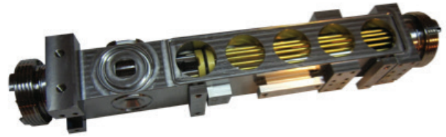
Deep Space Atomic Clock mercury ion trap housing with electric field trapping rods seen in the cutouts. This is where Deep Space Atomic Clock interrogates and measures the mercury ion resonance that is used to discipline a quartz crystal clock.
