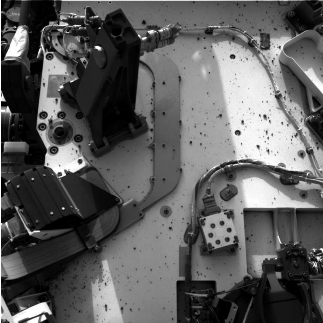
Figure 4.6.2-1 Particulates on the Mars Science Laboratory rover deck after touchdown.
