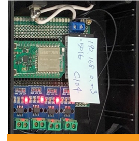
MediaTek LinkIt platform (MT7697 IC) used as smart IoT conference room sensing and status relay platform
