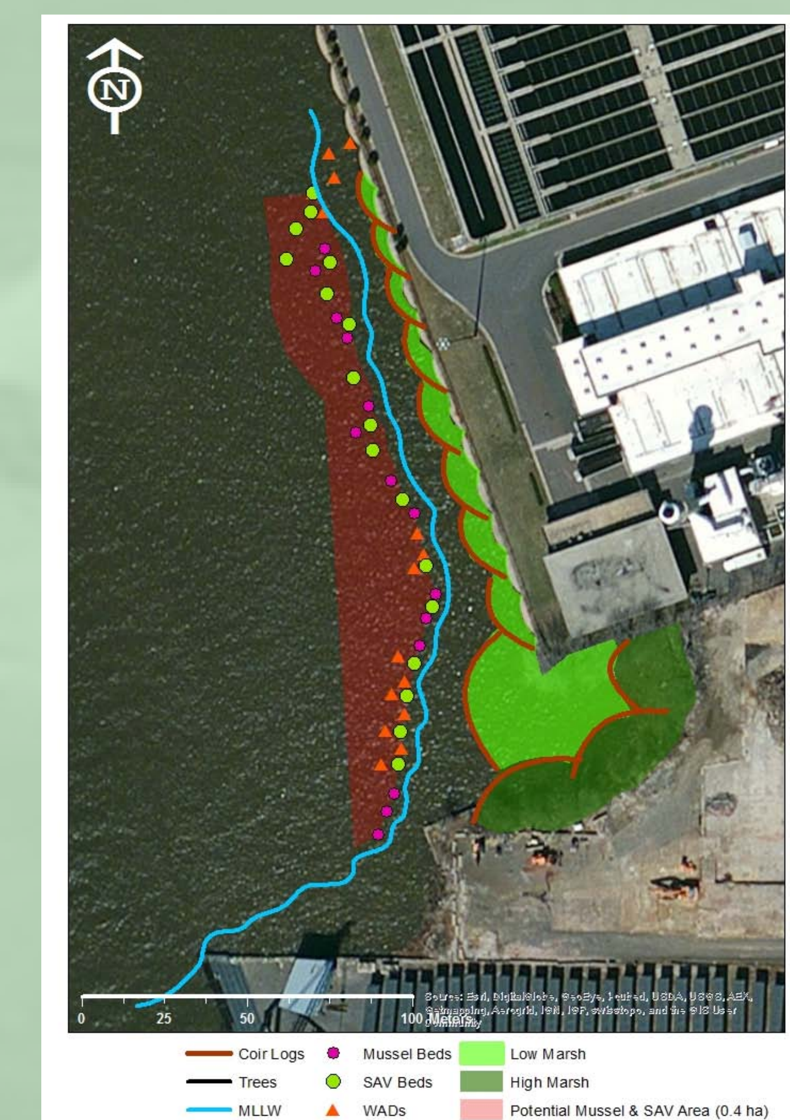
Figure 8. Conceptual diagram for a hybrid living shoreline at the Phoenix Park site in South Camden, New Jersey. The project would expand intertidal high and low marsh and encourage subtidal communities of SAV and freshwater mussels.
