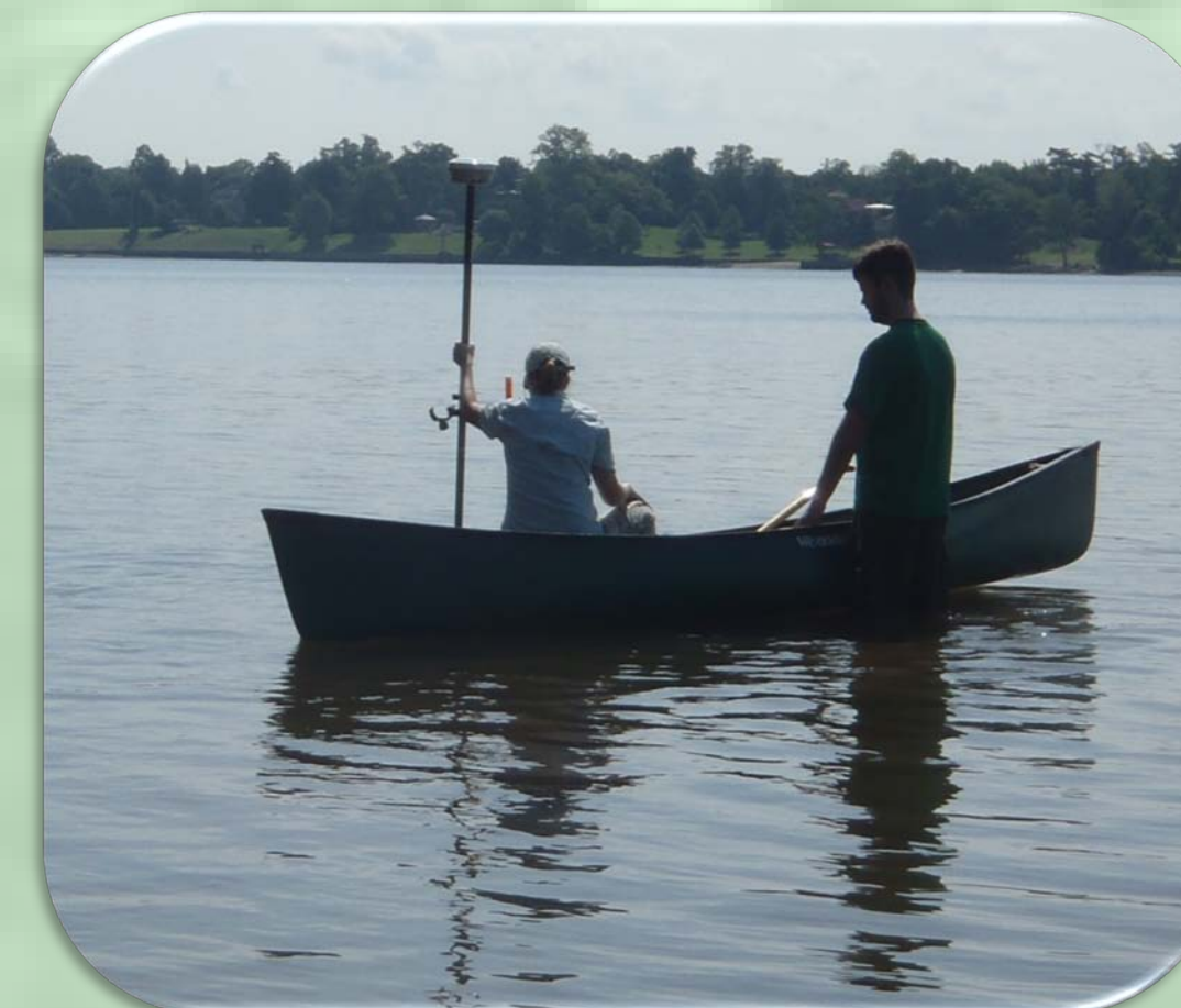
Figure 2. RTK-GPS surveys of intertidal and shallow subtidal elevations.
