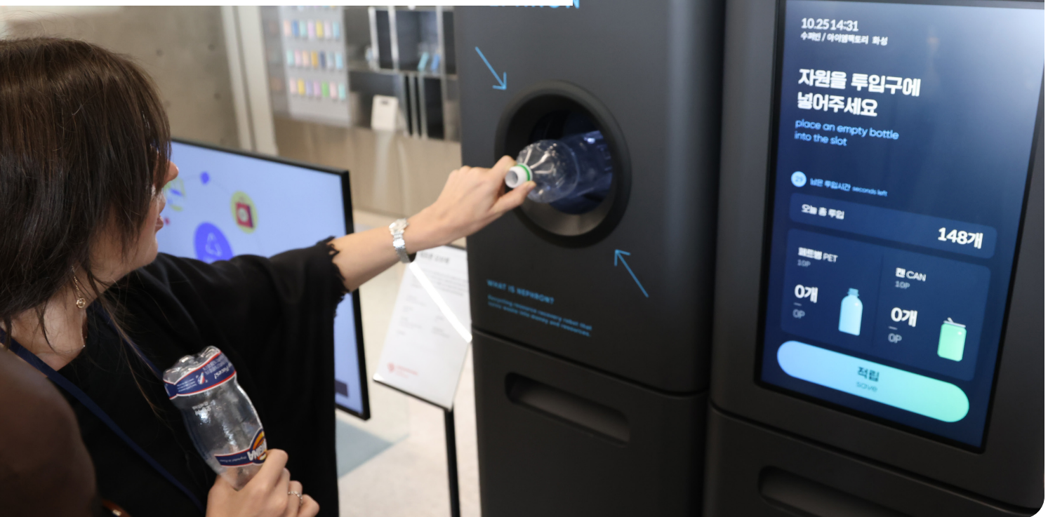
Photo: Woman demonstrates how to use plastic recycling vending machine. Study team.
