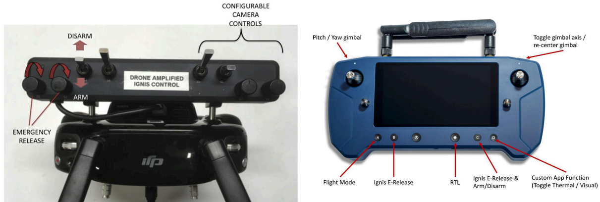
Figure 4.1.7: Left: Ignis control switches for the M600. Right: Ignis control switches for the Alta X and IF 1200.
