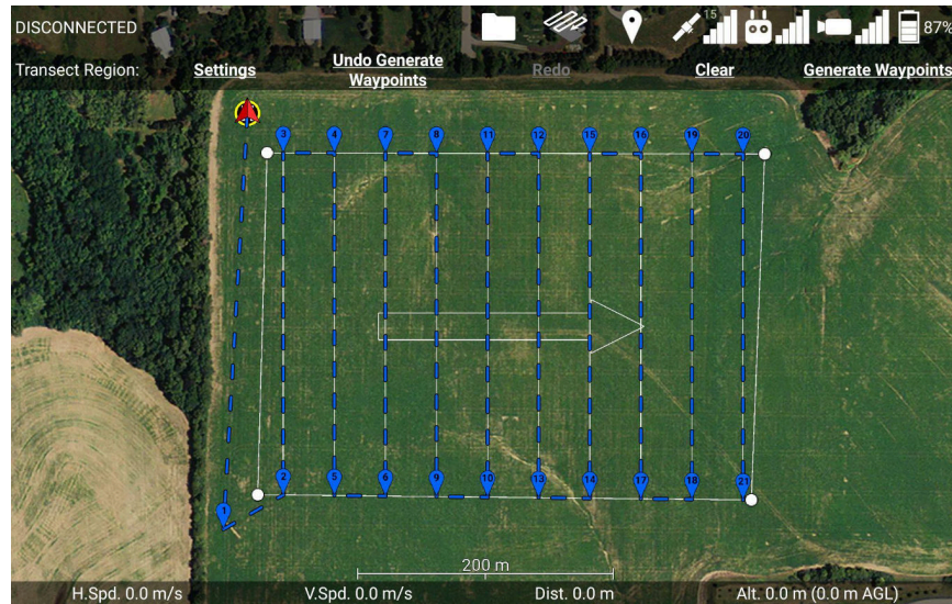
Figure 7.16e: The generated waypoints of the transect region will start near the end of the ingress route.
