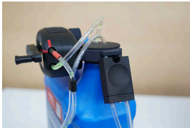
Figure 1.11c The coupler stores on the front of the pump mounting bracket when not in use.
