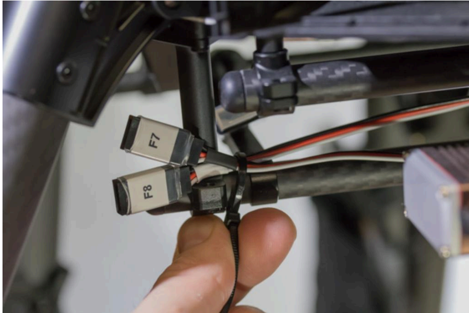
Figure 9.2f: Ziptie the connectors in place.
