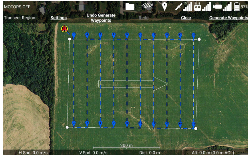
Figure 7.16c: Touch the Generate Waypoint button to generate waypoints that follow the transects.
