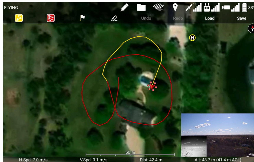
Figure 7.18.1: Using the drone to draw a line on the map. The color was changed from red to yellow mid-way through.
