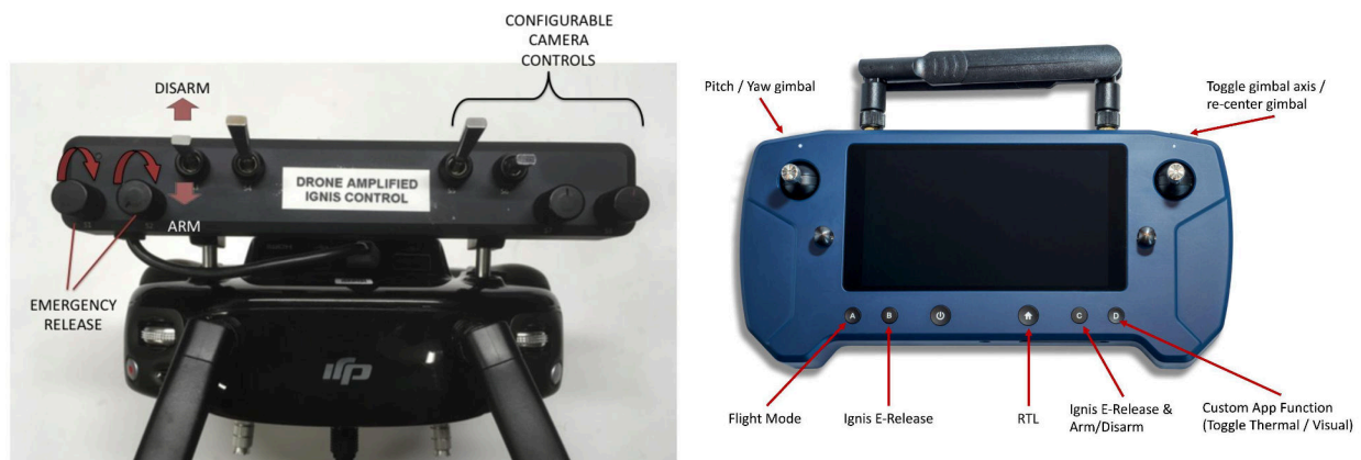
Figure 4.1.15: Left: Ignis control switches for the M600. Right: Ignis controls for the Alta X and IF 1200.
