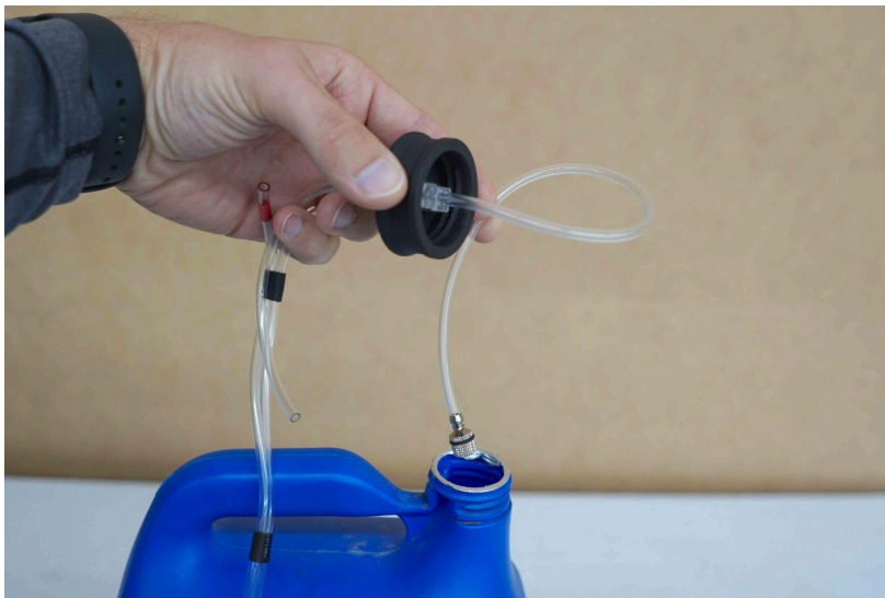
Figure 1.11a: Put the pickup clunk and tube into the jug first and tighten the cap.
