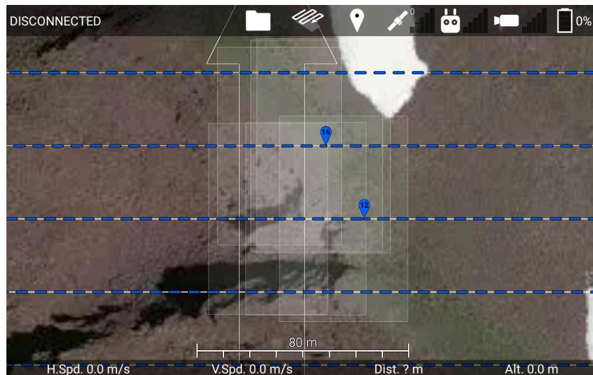
Figure 7.16.2c: After adding intermediate waypoints from the side view, the photos overlap the correct amount.
