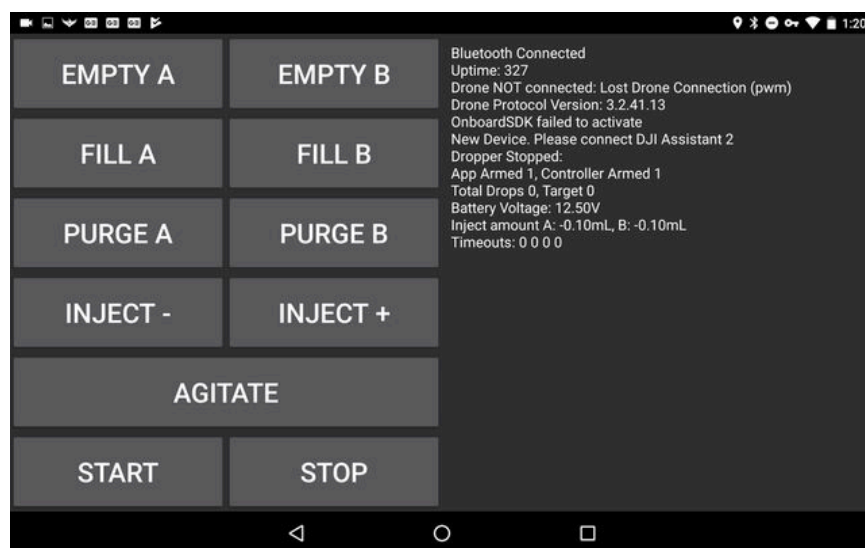
Figure 9.4a: Error message displayed when the Matrice 600 has not performed the DJI Onboard SDK Activation with Ignis.
