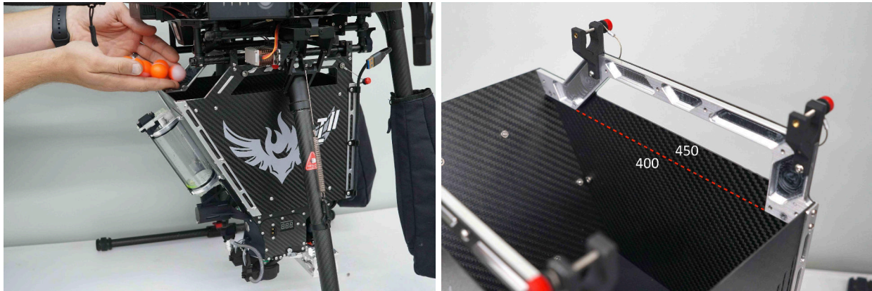
Figure 4.1.12: Left: Filling the Hopper with ignition spheres. Right: Approximate capacities.
