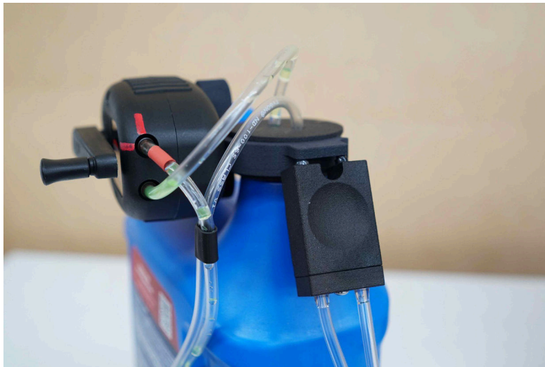
Figure 4.1.13d: Store the coupler on the antifreeze jug between uses to prevent contamination from dirt and to prevent siphoning.
