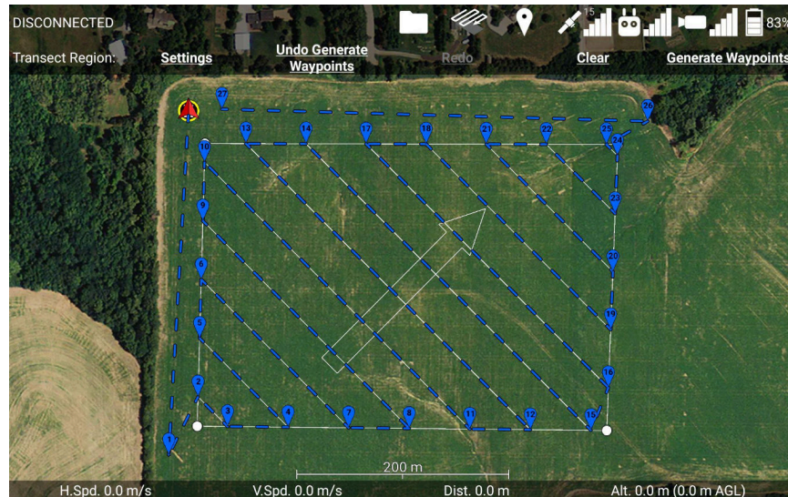
Figure 7.16g: Generating waypoints again will replace the part of your waypoint mission that passes through the transect region.
