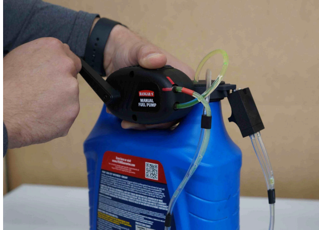
Figure 4.1.13a: Prime pump by cranking rapidly clockwise until antifreeze enters the pump.
