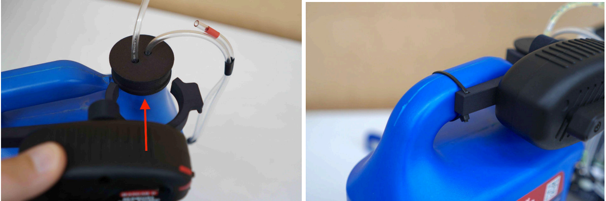
Figure 1.11b: Snap pump mounting bracket on the cap and zip-tie the other end to the handle.
