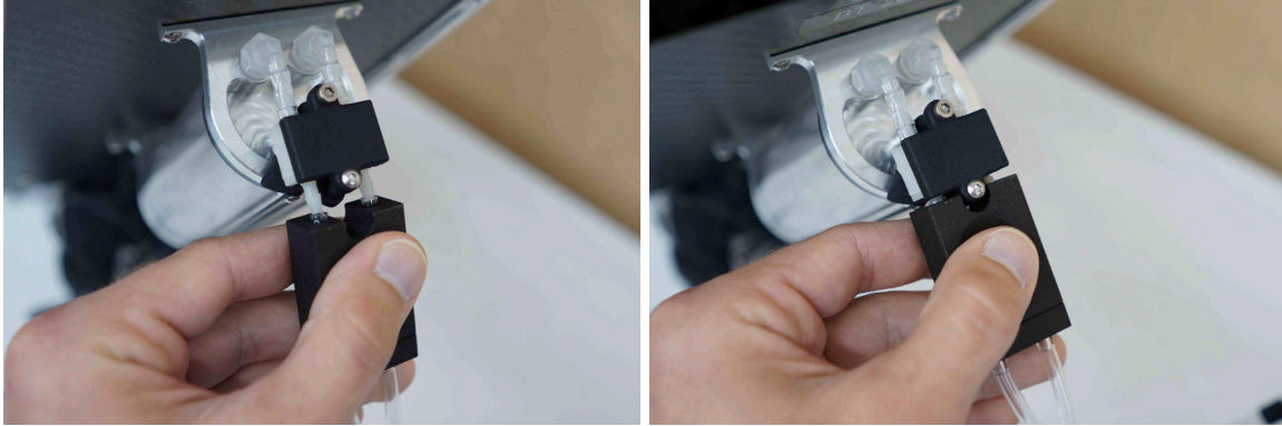
Figure 4.1.13c: Left: Align the tubes on the coupler with the check valve barbs. Right: Press the coupler onto the reservoir until it stops.
