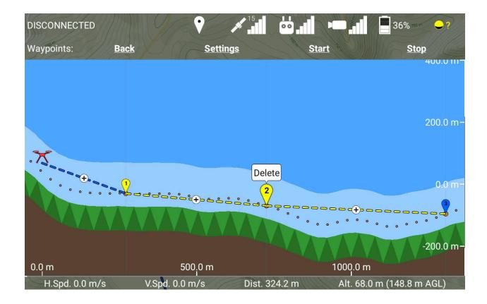
Waypoints that are colinear (or nearly colinear) with their neighbors can also be dragged left and right in the side-view, which corresponds to moving them closer to the previous waypoint, or closer to the next waypoint. This works nicely with the + button, so you can drag the new waypoint exactly where you want it.
