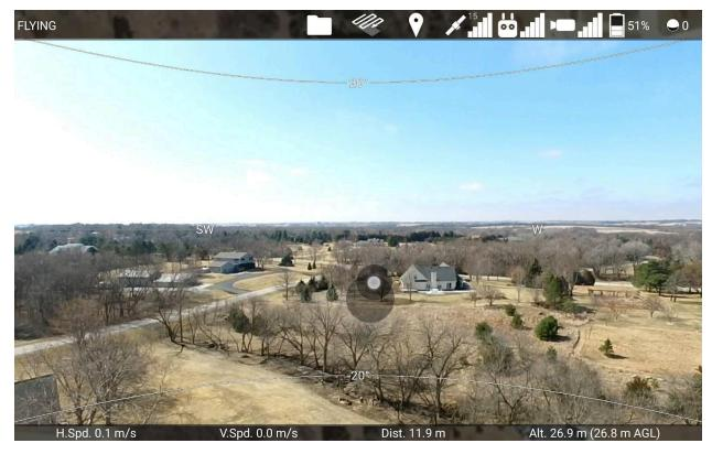
It's like the camera is centered inside a sphere that has lines drawn around it at 0, 20, 40, 60, and 80 degrees of pitch. It's easy to understand how far up or down the camera is pitched just by looking at the curvature of the lines. Additionally, compass directions like N, NE, E, SE, etc. are written along the 0 degrees pitch line.
