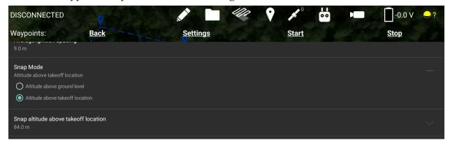
In previous versions of the app, and by default, the setting is set to Altitude above ground level, which lets you easily make terrain-following missions like this:
