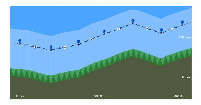
The new setting makes the snap line flat so you can easily make missions where the drone doesn't ascend or descend.
