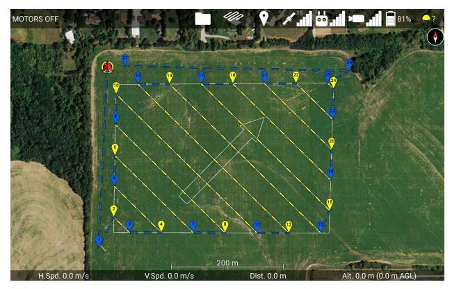
Touch the zig-zagging arrow icon at the top of the screen, to open the transects menu, then touch the map at the corners of the area you want to fly over. Adjust the transect settings to configure the angle and spacing of the transect lines, then touch the "Generate Waypoints" button to generate the waypoints.
