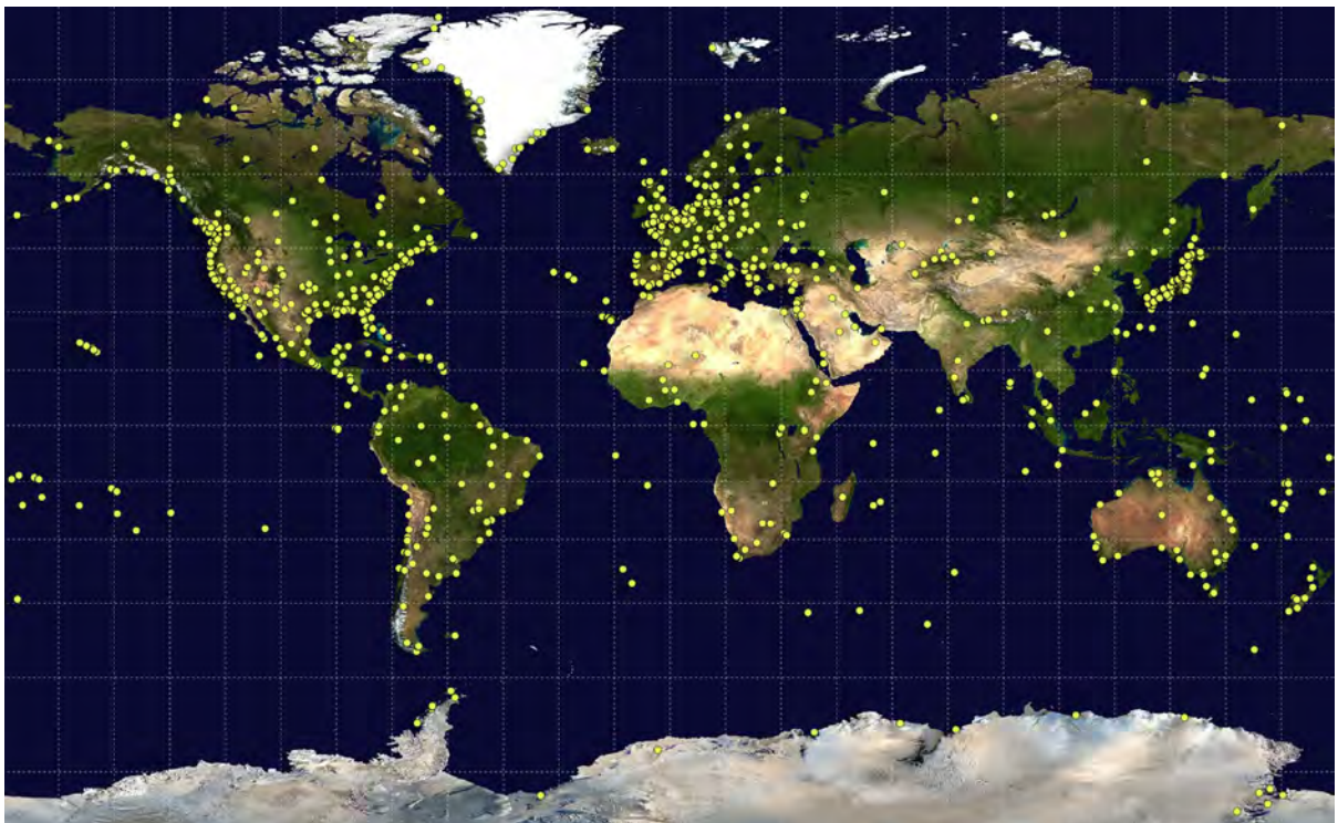
Figure. Sites around the world (yellow dots) contributed data and serve as “landmarks along a trail” for the newest update to a global standard called the International Terrestrial Reference Frame. Each site conducts precision measurements using at least one and up to four of the geodetic techniques described in this article. Image credit: GSFC/Earth Observatory
