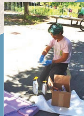
Cy David coats a machined foam hillslope with sand to improve flow.
