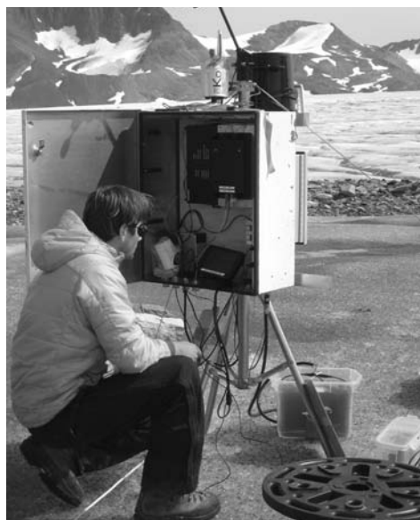
EPS Graduate student Leif Karlstrom installing a Distributed Temperature Sensor on the Mendenhall Glacier, AK
