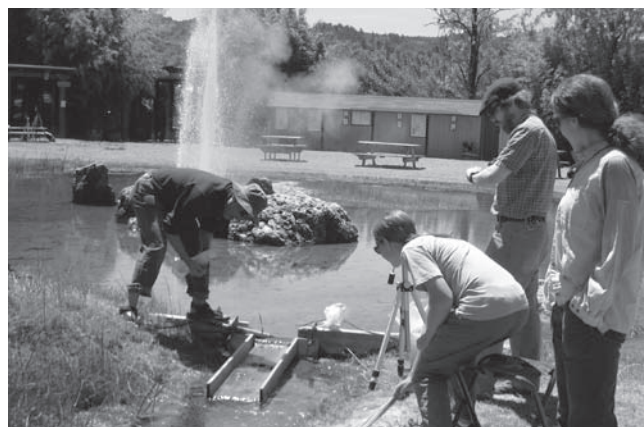
A scene from the Calistoga experiment showing the measurement of the discharge from a pool around the Calistoga geyser. Standing are two EPS graduate students, Ben Andrew and Jennifer Frederick, and USGS scientist Darcy McPhee. The wooden weir was constructed at our department machine shop by John Werner.
