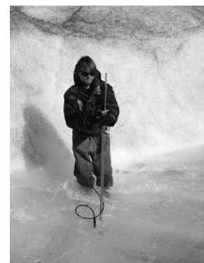
Adam Zok, making discharge measurements in a supraglacial stream on the Mendenhall glacier, Alaska.
