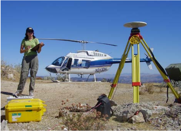
Roland Bürgmann's graduate student Kelly Grijalva sets up a GPS receiver at a site in the San Benito Mountains, which required the use of a helicopter for access. These measurements are used to characterize deformation along the creeping segment of the San Andreas fault.
