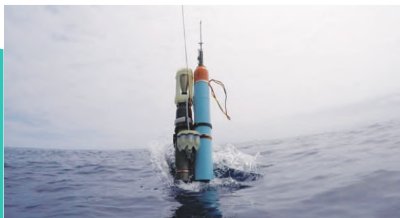
The system shown in the photograph above—constructed mostly from 3D printed parts fabricated in Jacobs Hall—went from design to the ocean in less than one month. The study which took place in California coastal waters in August 2016 R/V Oceanus (photo by Jessica Kendall-Bar) and June 2017 aboard R/V Revelle.
