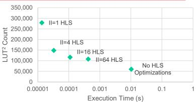
Rapid design space exploration in geolocation HLS design by "tweaking" HLS initiation interval (II) parameter
