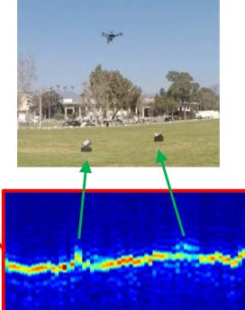
Results of Flight Demonstration. Radargram shows the surface return as well as the presence of two small corner reflectors.
