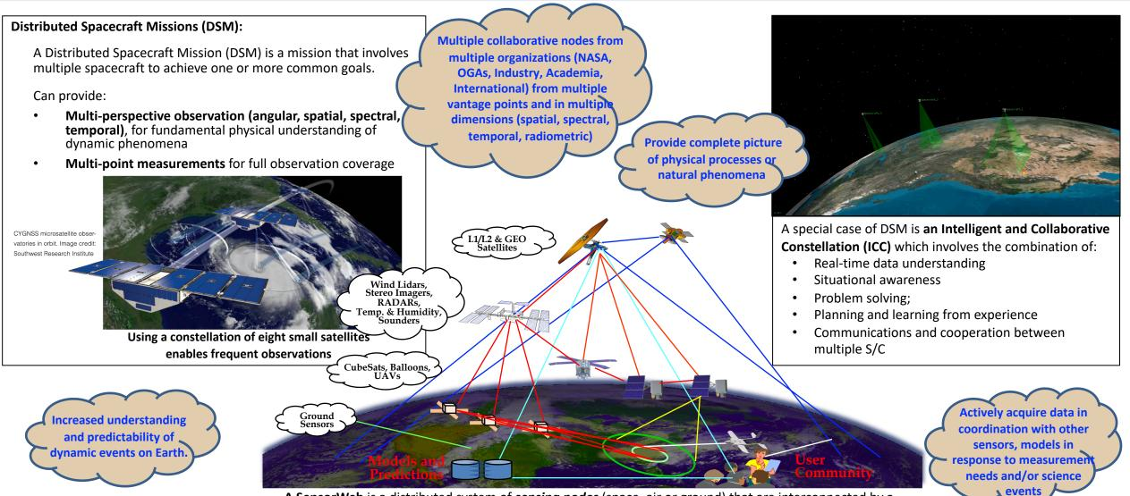
A SensorWeb is a distributed system of *sensing nodes* (space, air or ground) that are interconnected by a *communications fabric* and that functions as a single, highly coordinated, virtual instrument.
