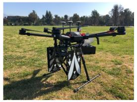
UAV with SDRadar mounted
