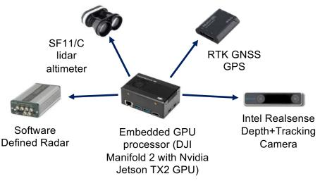
Next generation UAV-SDRadar sensor payload
