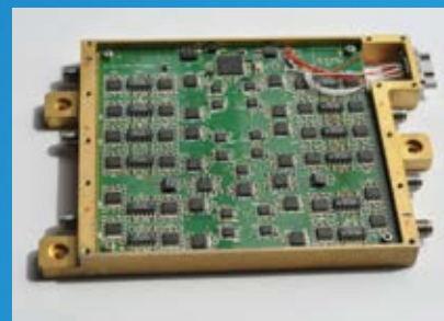
A mixed-signal printed circuit board for the intermediate frequency processor module developed as part of the ACT project. Credit: W. Blackwell, MIT
