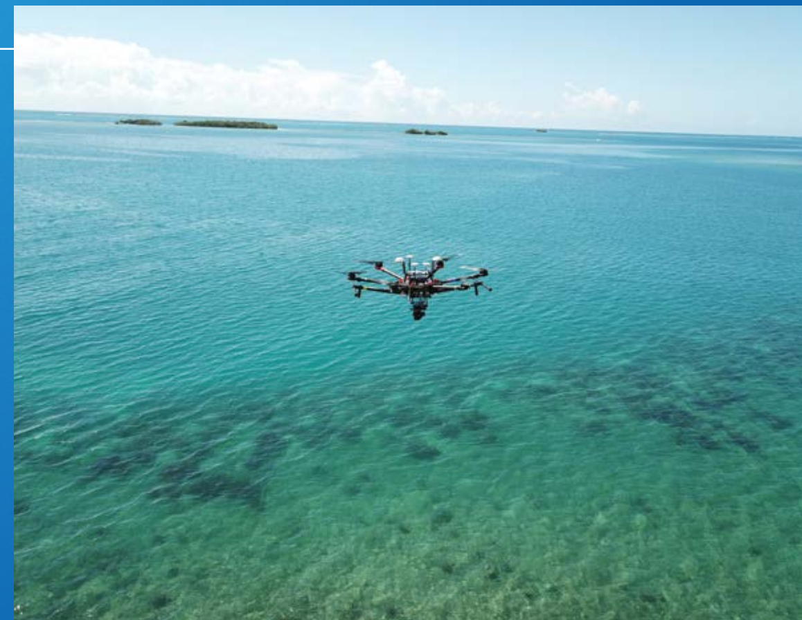
↪ A small drone equipped with FluidCam observes a coastal seabed. FluidCam, Fluid Lensing, and NeMO-Net provide researchers with clear, undistorted images of the ocean floor, making it easier to study coral reefs. Credit: Ved Chirayath / NASA Ames
