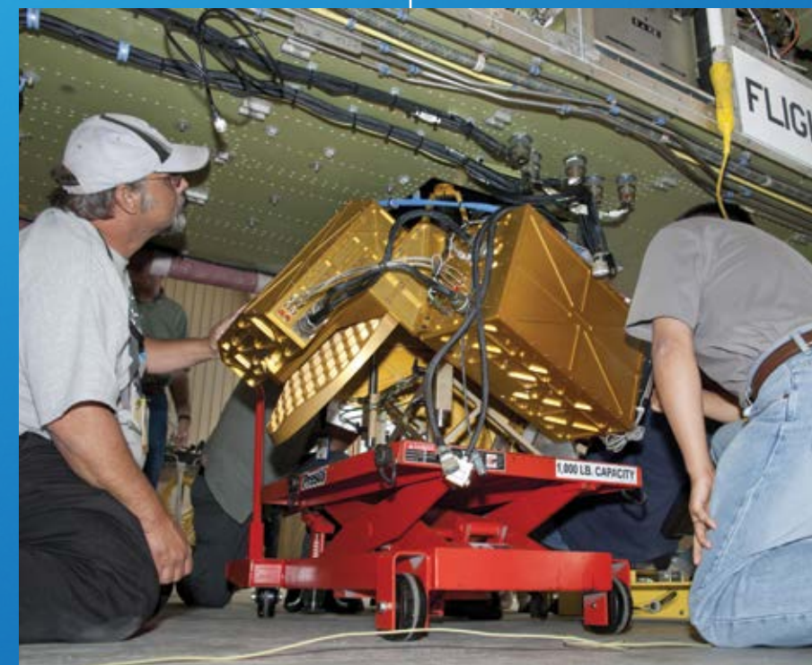
Technicians install HIWRAP on the underside of a NASA Global Hawk in preparation for the GRIP campaign in 2010. Credit: Tony Landis / NASA
