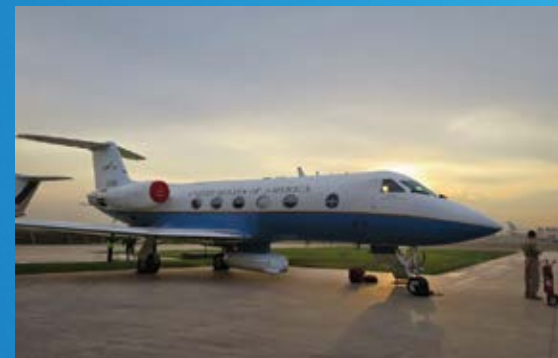
From 2014, the UAVSAR radar pod mounted below the NASA Gulfstream-III jet. Credit: JPL
