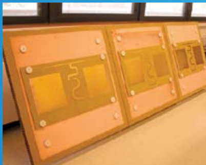
The full-scale dual-frequency feed array developed under the MOSS project. Credit: M. Moghaddam / University of Michigan
