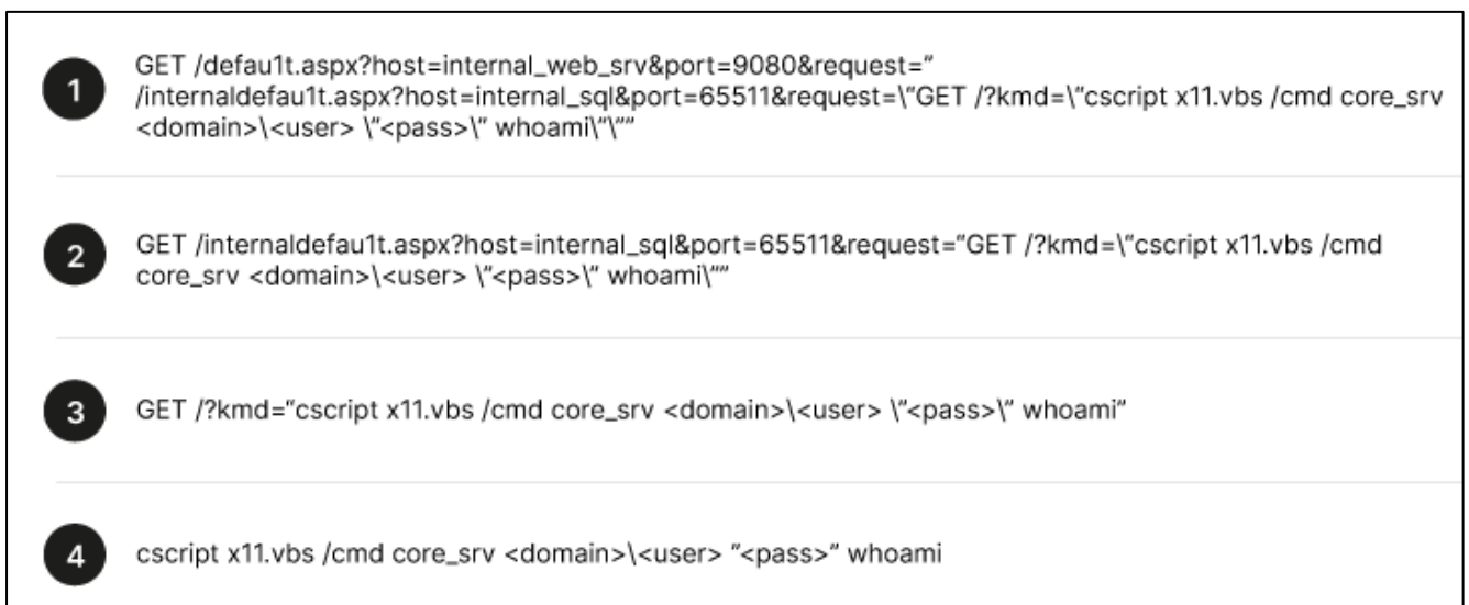
Figure 18: The decapsulation of the HTTP requests sent for executing WmiExec.vbs on a core server via the PowerShell backdoor on the SQL instance, ordered by the stages on Figure 17.
