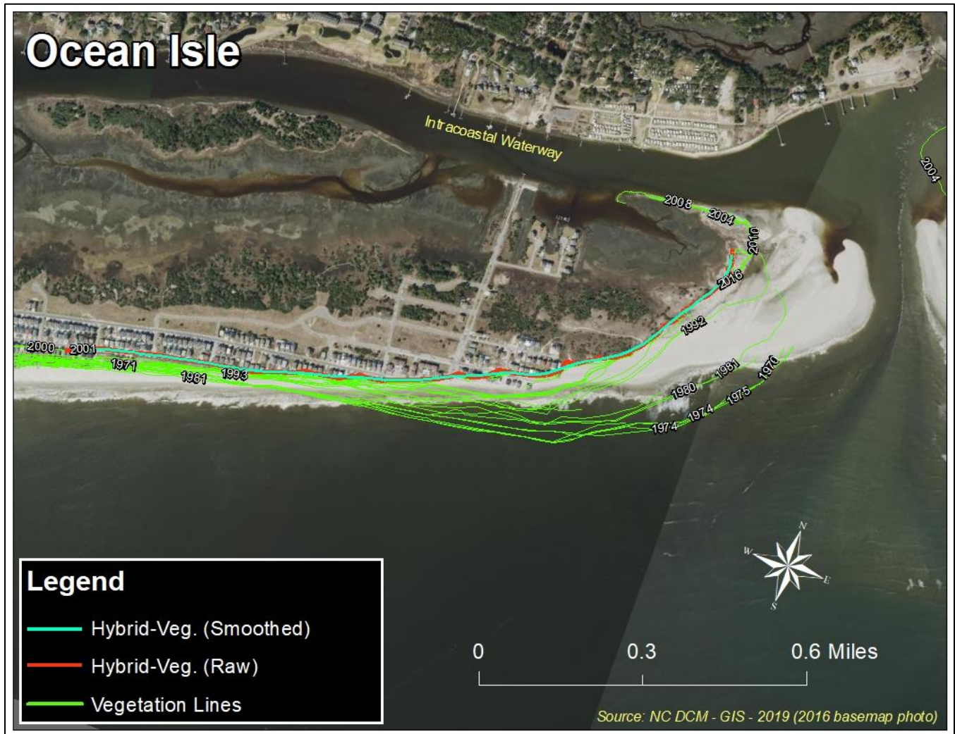
Figure 15. Shallotte Inlet at Ocean Isle. Vegetation Lines mapped: 1970, 1974, 1975, 1980, 1981, 1987, 1990, 1992, 1993, 1998, 2000, 2001, 2003, 2004, 2008, 2009, 2010, 2012, 2016. Vegetation line segments making up the Hybrid-Vegetation Line: 1998, 2000, 2001, 2003, 2004, 2008, 2009, 2010, 2012, 2016.
