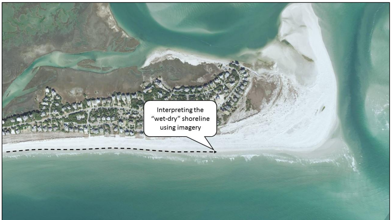
Figure 4. Interpretation of the "wet-dry" shoreline using orthophotography.
