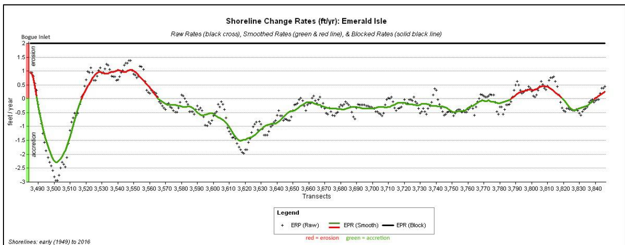
Figure 53. Emerald Isle shoreline change rates and blocked rates (setback factors). Black-points represent all (erosion and accretion) raw rates; smoothed rates are represented by the solid green (accretion) and red (erosion) line; and the solid black line represents blocked rates (setback factors).
