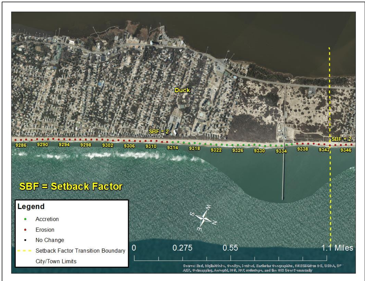
Figure 93. Duck shoreline change rates and blocked rates (setback factors). Black-points represent all (erosion and accretion) raw rates; smoothed rates are represented by the solid green (accretion) and red (erosion) line; and the solid black line represents blocked rates (setback factors).
