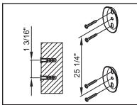
(1) Drill four 1/4" holes as shown in the drawing. Using hammer to tap plastic anchors into the holes and flush with the wall. Secure the mounting plates on wall with help of mounting screws. Make sure two mounting plates are 25-1/4" apart
