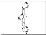
(3) Place slide bar to bottom mount. Place bottom mount on mounting plate. Tighten mounting screw on the side of bottom mount. Align the notch on the bottom of slide bar so the notch faces back on bottom mount. Tighten Allen screw by using 3/32" Allen wrench.
