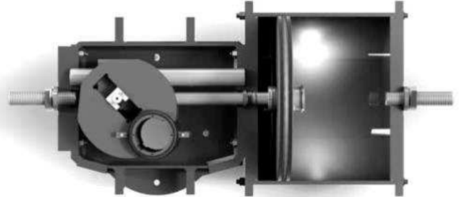
Figure 20: Double Acting Actuator Configuration – Open Position
