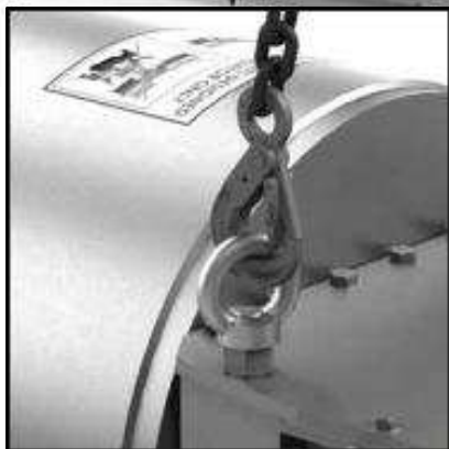
Figure 3: Use of Eyebolt on the Scotch Yoke Housing Cover
