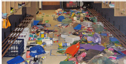
Fallen contents in classroom
