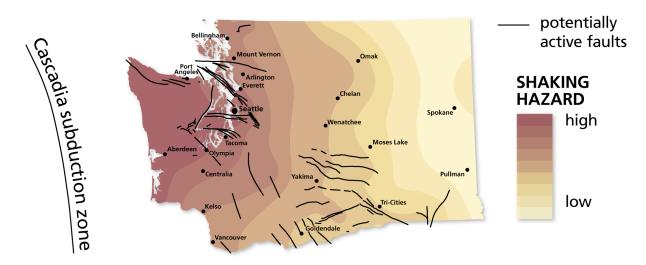
**Figure 5.** Map of the seismic hazard in Washington State, expressed as contours of peak ground acceleration (anticipated ground shaking, or acceleration in bedrock) as a fraction of standard gravity. These values are from the USGS two percent probability of exceedance in 50 years map of peak ground acceleration, which is a proxy for shaking hazard (Peterson and others, 2015). Warmer colors indicate higher hazard areas. Major active faults are shown as black lines.
