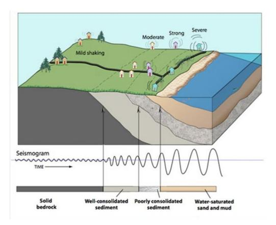
**Figure 7.** Schematic figure illustrating how seismic waves travel through different rock and soil types. The type of rock or soil beneath a structure greatly affects how a building responds to earthquake shaking. Geologists measure the time it takes sound waves to travel through the ground at each school campus to determine the rock/soil type and correlate it to a site class value. This value is then incorporated into the engineering assessment. https://slideplayer.com/slide/6132863/
