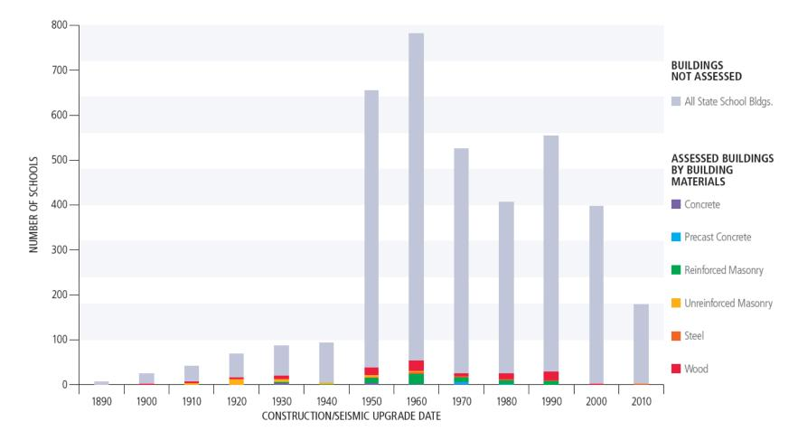
**Figure 22.** Histogram of the number of permanent, public K–12 Washington schools (gray) categorized by decade built or the date there was a last major seismic upgrade based on the ICOS database. Schools assessed in Phase 1 are colored by construction type (such as wood and concrete).
