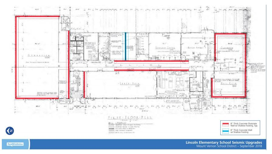
Figure 17. Example of a seismic upgrade design plan for part of the first floor of Lincoln Elementary School, Mount Vernon, WA.
