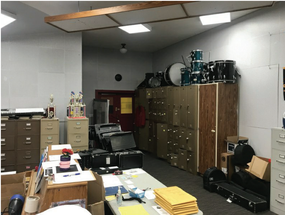
Figure 1-3. Band room with unsecured storage units and heavy instruments stored on top of units.
